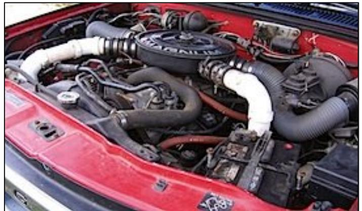
Fig. 4: PVC piping directs cooled and filtered woodgas to the engine.
