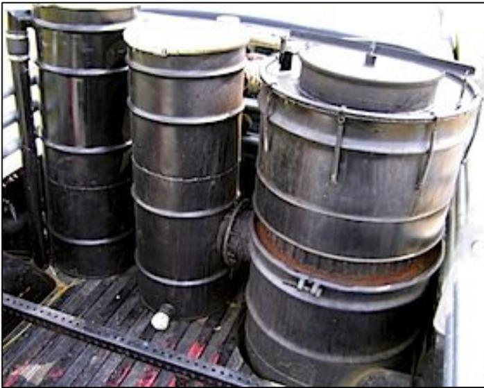
Fig. 4: from right: gasifier, heat exchanger, filter.
